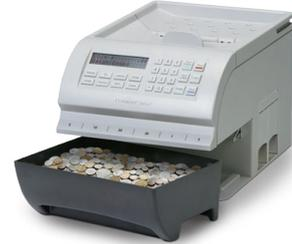
**Value Counter Option:** All coins are counted by denomination and collected into a single transfer box, which is easy to pour into a larger central JetSort for consolidated processing.
